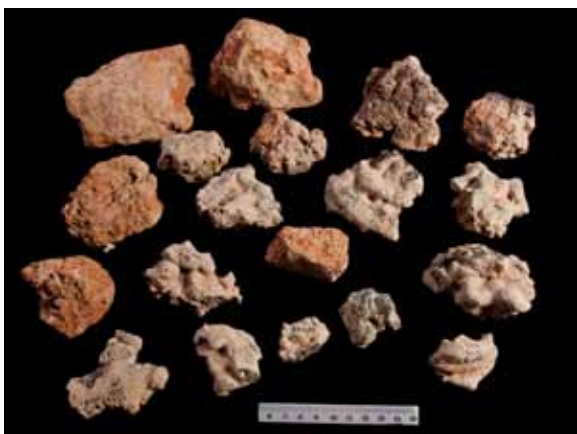
Fig. 2.16. Clay lumps and slag from the pottery kiln and adjacent areas.
